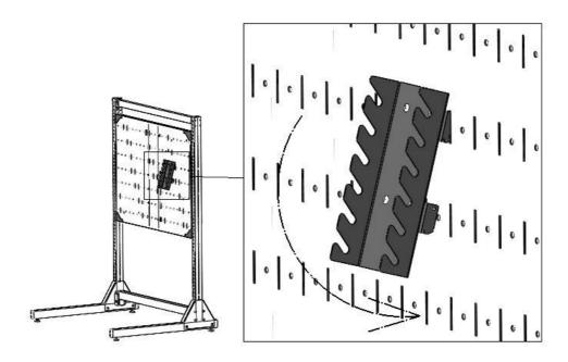
Step 3: After straightening, Pull down the Spanner tray to properly fit it in the Slot.
