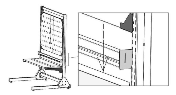
Option 2: To use bin rail in Inclined position (Position 2), don't use the upper notch; use the rear hook of the bracket and lower notch of bin rail as shown in the below image.
