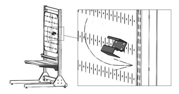
Step 3: After straightening, Pull down the Allen key holder to properly fit it in the Slot
