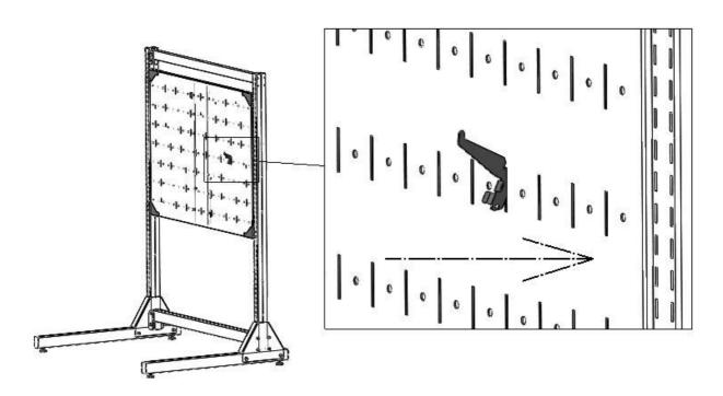
Step 2: Straighten the hook to a vertical position.
