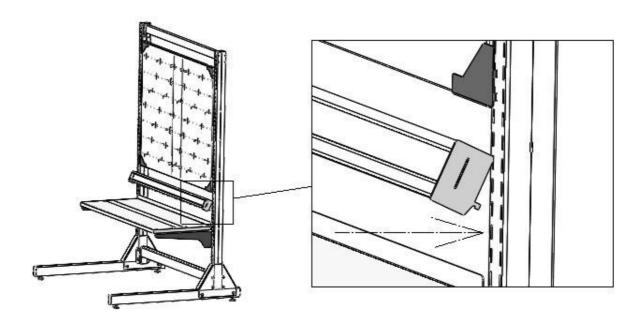
Step 2: After inserting it in the Slot of the Pegboard panel, straighten the Bin rail as shown.
