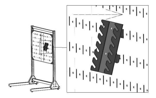
Step 2: After inserting the Spanner tray into the slot of the Pegboard panel, align and straighten it as shown.
