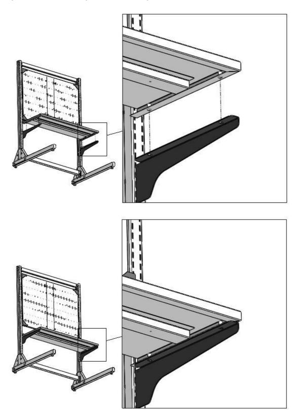
Step 4: Fasten the Shelf body to Mounting brackets using M6X15 Allen dome head screw.
