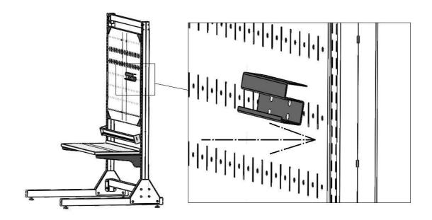
Step 2: After inserting the Screw driver holder into the slot of the Pegboard panel, align and straighten it as shown.
