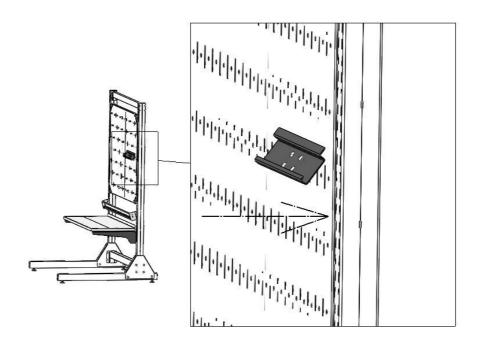
Step 2: After inserting the Bin strip into the slot of the Pegboard panel, align and straighten it as shown.
