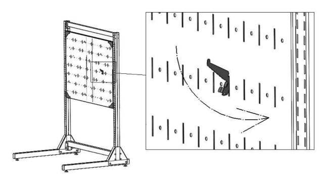
Step 3: Pull down the hook to lock it securely into the slot.
