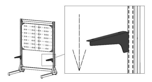
Step 3: Align the Shelf body holes and Bracket holes as shown in the below image and place the shelf on top of the mounting bracket.
