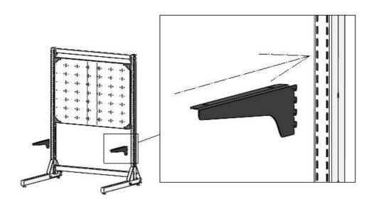
Step 2: Pull down the bracket after inserting it in Link uprighter slots for proper fitting.
