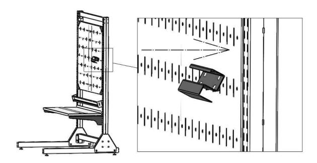
Step 2: After inserting the Allen key holder into the slot of the Pegboard panel, align and straighten it as shown.
