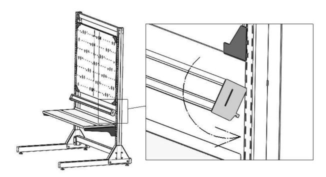
Option 1: To use bin rail in Straight position (Position 1) use upper notch and lower notch as shown in below image.
