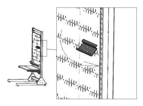
Step 3: After straightening, Pull down the Bin strip to properly fit it in the Slot
