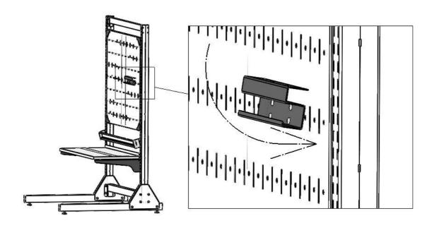
Step 3: After straightening, Pull down the Screw driver holder to properly fit it in the Slot
