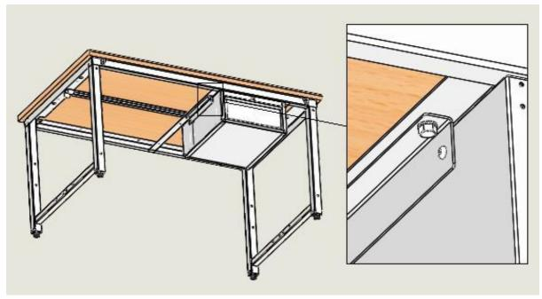
Step 7: Fasten the inserted bolt using an M8 Locknut.
