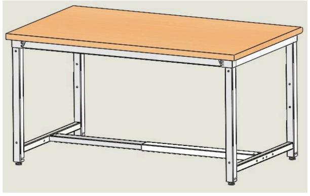
Step 4: Fasten the Inner and Outer channel with the Mounting brackets using M6X12 Allen dome head screw.
