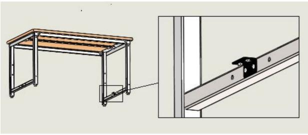
Step 3: Insert the inner channel inside the outer channel and place it on top of the mounting bracket assembly, matching the oblong holes on the channel with the M6 Weld nut provided in the mounting bracket assembly.
