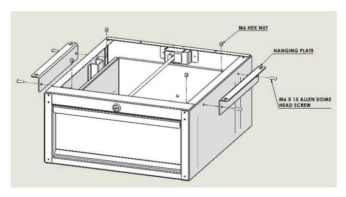
Step 5: After assembling the hanging plate with the hanging cabinet body, align and position the oblong holes of the hanging plate with the holes in the side mounting angles.
