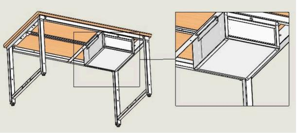
Step 6: Insert an M8X1.5mm Thick Washer into an M8X20 Hex Bolt, and insert both into the side mounting angle through the hanging plate, as shown in the image below.
