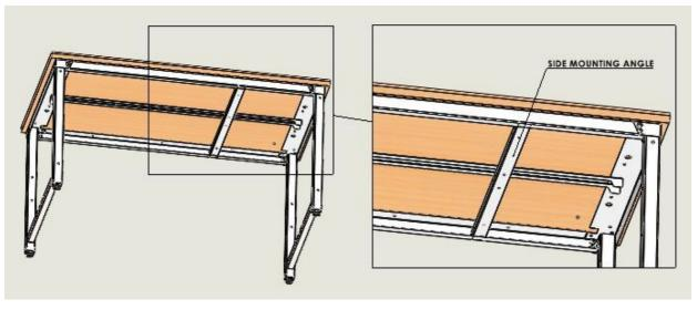
Step 3: Insert another side mounting angle using the same procedure, but with the opposite orientation.
