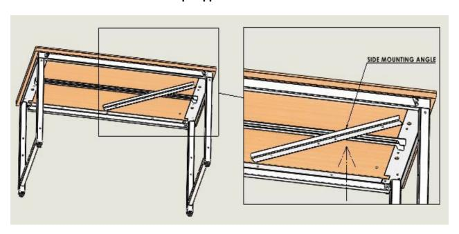
Step 2: Straighten the Side mounting angle after inserting between top support rail as shown.
