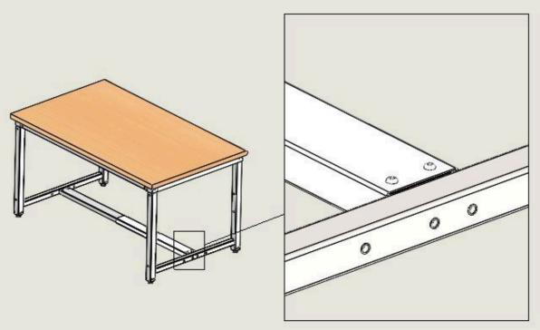
Step 5: Align the slots on the outer channel with the holes on the inner channel as required, and fasten them using M6X12 Allen Dome Head Screws and M6 Hex Nuts.
